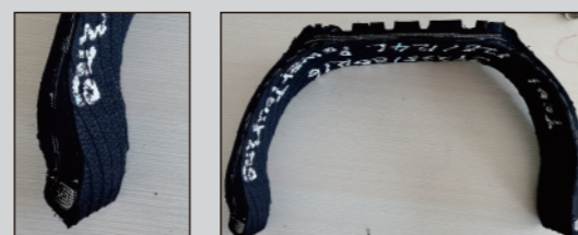
2-PLY Polyester Construction (ST235/85R16 with 3-PLY Polyester)
